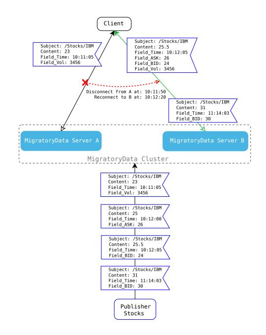
Figure 5.6: Example of Data Recovery With Standard Message Delivery Enabled
